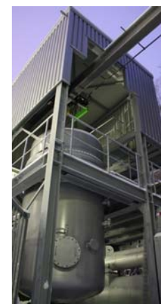
Test rig "HOTREG" for high-temperature regenerator storage at DLR
