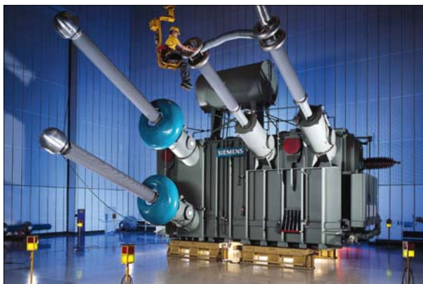
Fig. 3: Siemens has built several GW of high-voltage DC transmission lines worldwide. This is a 235-MVA-HVDC power transformer for the Australia-Tasmania undersea cable. An even larger line is being built in China (1400 km with a power transmission capacity of 5 GW). Photo: Siemens
